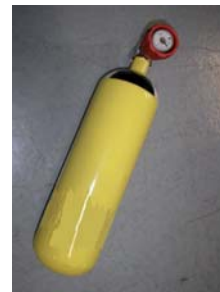
2-liters air bottle at 200 bar. Pressure reducing valve pre-set at 15 bar and extension lead
