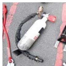
Air bottle at 4.350 PSI- pressure reducing valve pre-set at 210 PSI and extension lead
